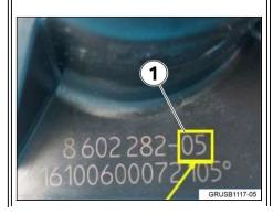
Check the index number (1) on the new thermostat (PN 11 53 8 602 282). Improved service parts have an index number
