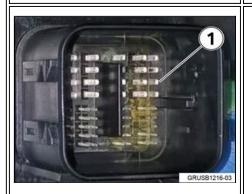
3. Check the DME and PDM connector sockets for coolant contamination (1).
