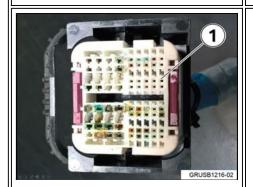
2. Check the wiring harness connector at the DME for coolant (1).
