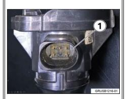
1. Remove the connector for the map thermostat (1) and check for coolant.
